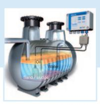
Application WGA 04 monitors oil, petrol and grease separators for accumulations of sand and sludge and generates an alarm signal when it is time to clean the separator. WGA 05 additionally monitors the thickness of the layer of separated liquid and generates an alarm signal when it is time to drain the separator.
