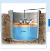
Application Together with the WGA-ÖW probe, WGA 06 monitors pump and control shafts in separator systems for oil accumulations and generates an alarm signal before pollutants can reach the sewage system. It is also possible to connect the WGA-AS probe. This way, the maximum levels in separators or retention tanks can be detected. This avoids overfilling that may be caused by clogged outlets or other circumstances. The unit keeps harmful substances from reaching the sewage water system.
