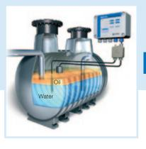
Application Oil, grease and petrol pose a great danger to groundwater and waste water. WGA 02 monitors the thickness of the layer of separated liquid in oil, petrol and grease separators and generates an alarm signal when it is time to drain the separator.
