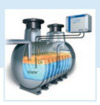
Application Oil and petrol pose a great danger to groundwater and waste water. WGA 01 monitors the thickness of the layer of separated liquid in oil and petrol separators and generates an alarm signal when it is time to drain the separator. In addition, the maximum level in the separator can be detected. This prevents overfilling that may be caused by clogged outlets or other circumstances. The unit keeps harmful substances from reaching the sewage water system.
