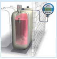
Application For continuous level measurement in tanks containing fuel oil EL, diesel fuel and other low-viscosity media which do not attack the materials of the indicator. For tank heights from 900 to 2,000 mm. The additional remote display enables convenient level indication even if the tank is not easily accessible. Suitable for remote measurements up to 10 m.
